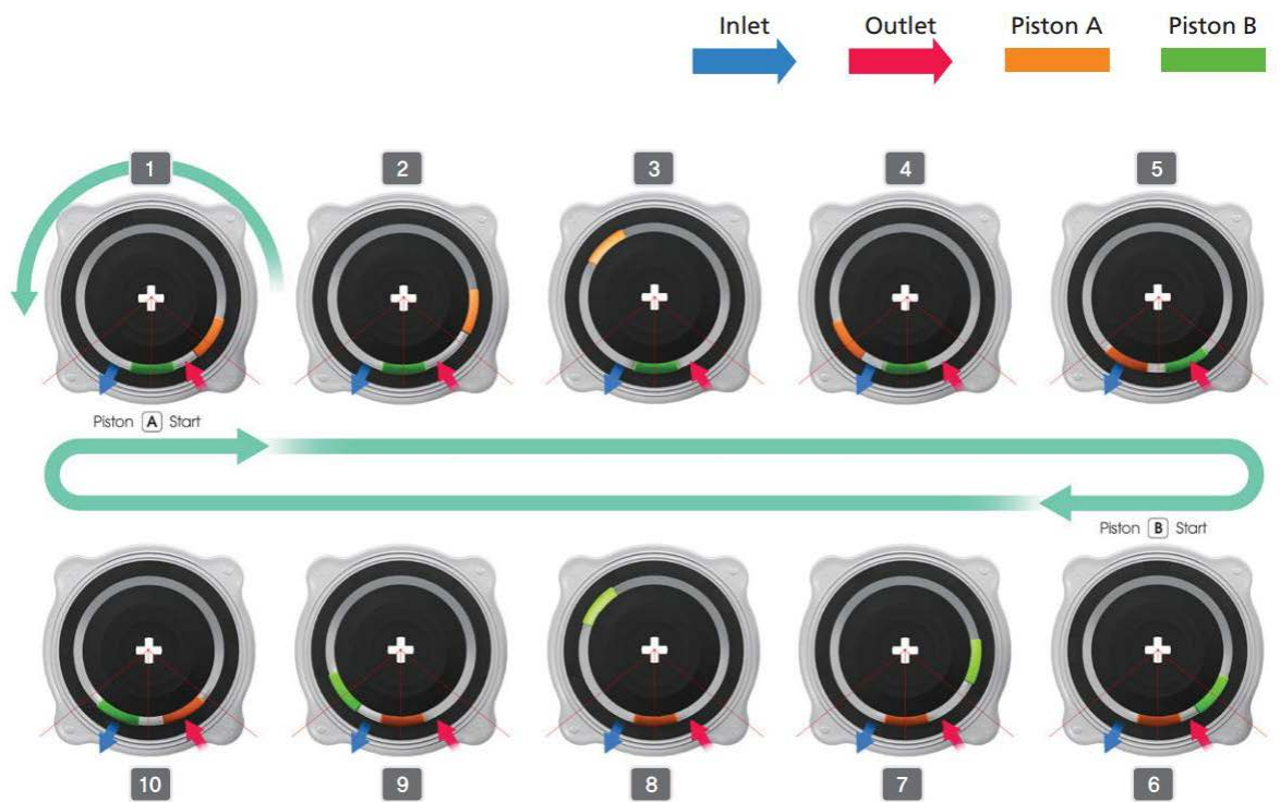
Figure 2. The mechanism of the Cylinder pump
